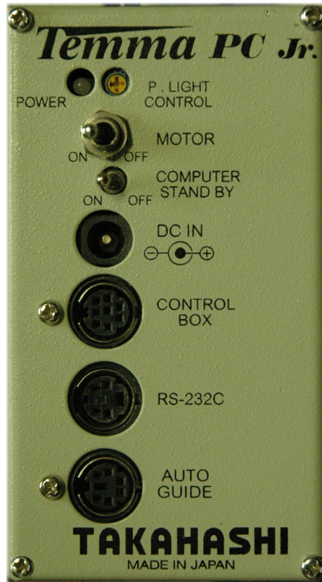
Figure 130: Temma PC Jr. Control Panel
