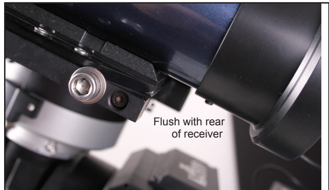
Fig 45: Position StarLock flush with the receiver.
