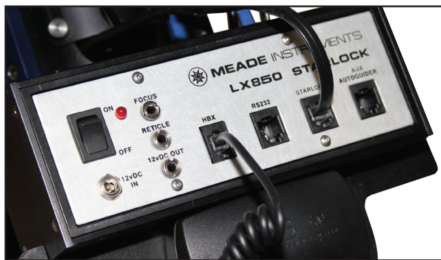
Fig 27: Connect handbox cable to HBX
