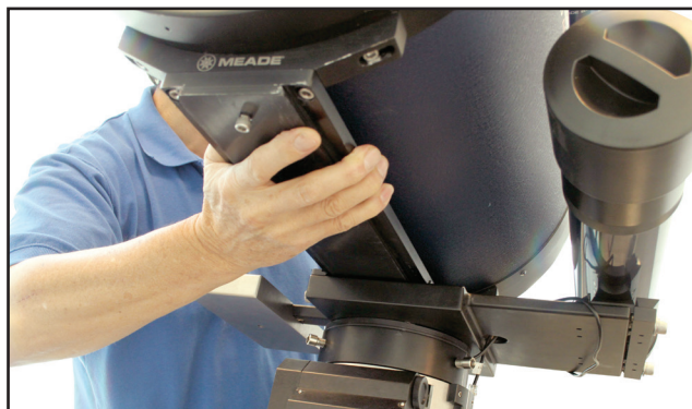
Fig 23: Slide the OTA dovetail into the saddle plate
