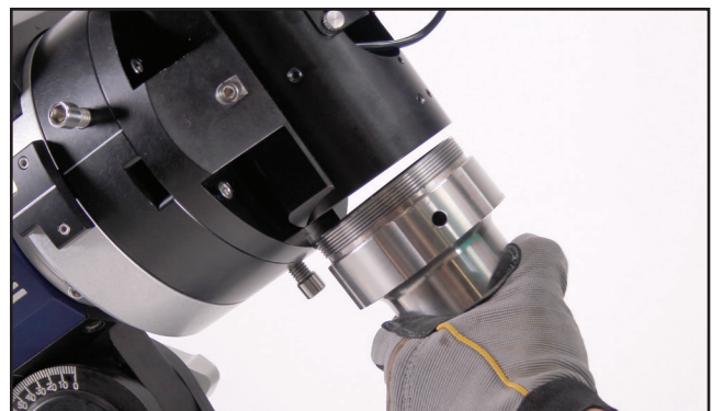
Fig 12: Attach Counterweight Shaft.
