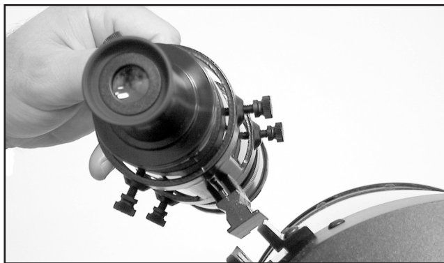
Fig 28: Slide viewfinder into receiver
